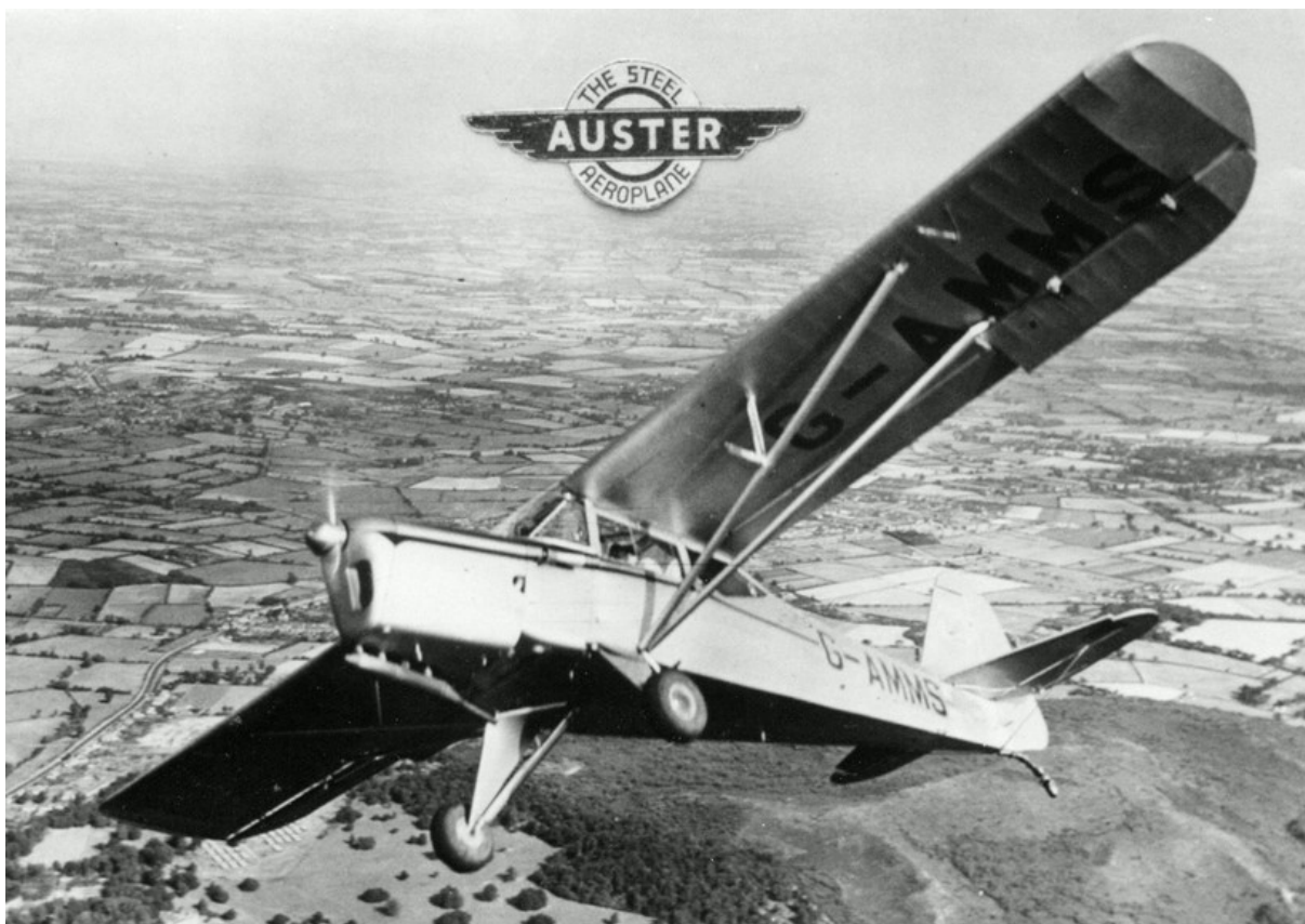
Auster's publicity shot of the Aiglet aerobatic trainer. This is G-AMMS which Ranald displayed at Farnborough in the 1950s. Note the extreme aileron deflection.
