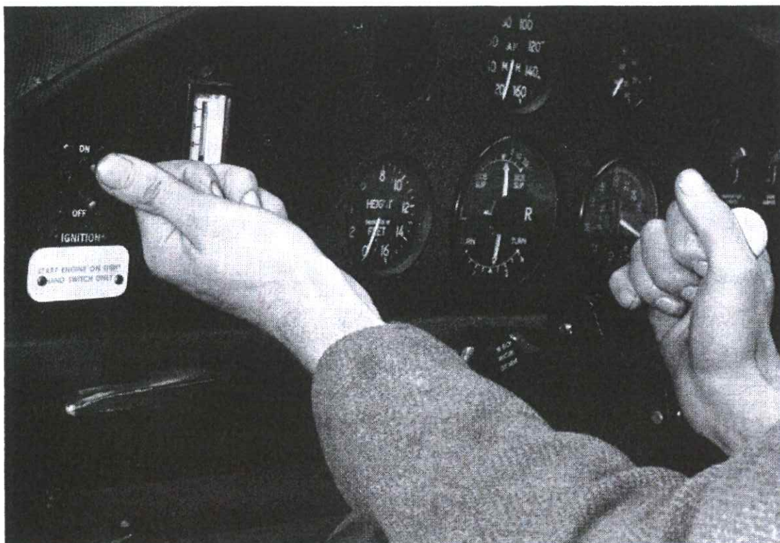
Figure 28.—When starting, the impulse starter is brought into operation by using the right-hand ignition switch.
