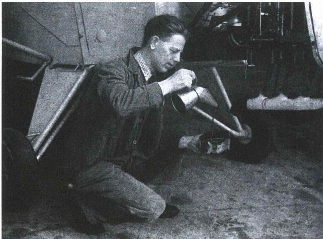
Figure 32.—Refill rocker box covers with oil to the correct level before replacing.
