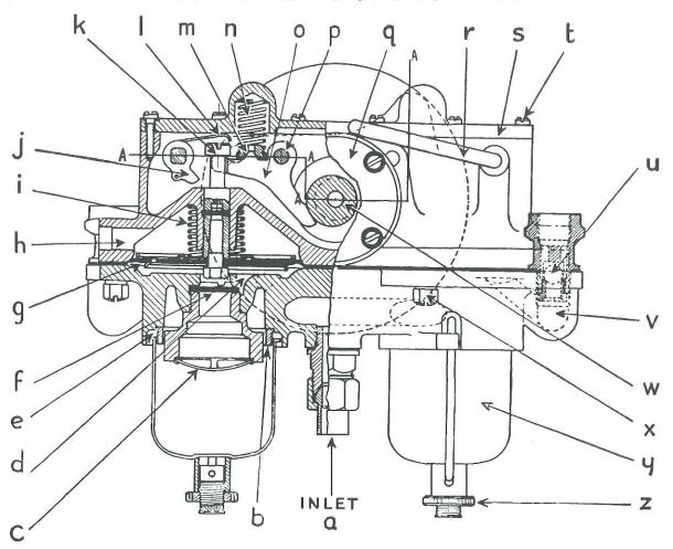
The pump is a self-contained unit attached to the engine by a flange. The drive is imparted by a rotary motion in either direction at half engine speed in accordance with the design of the engine maker. The pump as a unit has two sets of diaphragm pumps each independently operated, and although there is a common fuel feed inlet (a), each pump has its own filter, inlet valve and non-return outlet valve—the last named being coupled together externally to carry the fuel to the carburetter.
